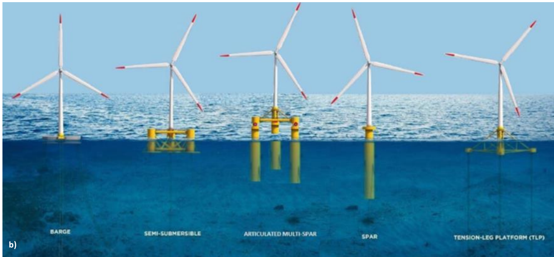
Figure 2.2: Offshore wind foundations a) Bottom-fixed and b) Floating [67][68]
