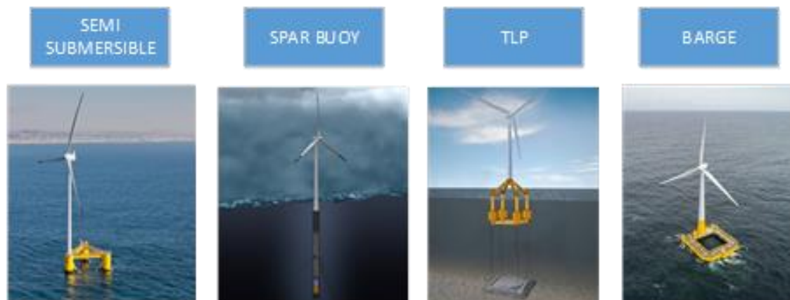
Figure D.7: Summary of floating wind platform technologies [286]
